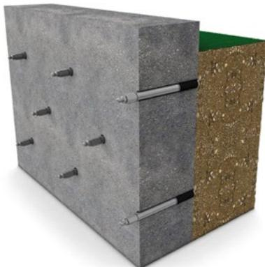
**Borepacker use:** Packer arrangement for concrete interfaces
