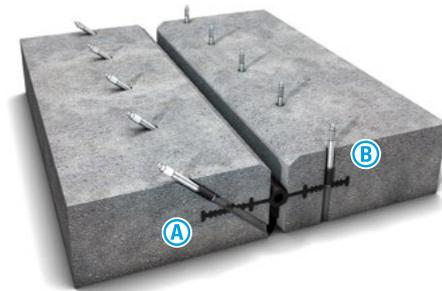
**Borepacker arrangement:** Drilled holes with inserted packers crossing construction joints through the joint strip flange. Techniques **A+B**
