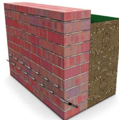
**Borepacker use:** Packer arrangement for masonry
