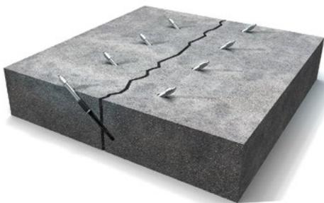
**Borepacker drill hole packers:** These are inserted in the drilled holes at a distance corresponding to half the crack depth in a staggered formation on both sides of the crack (usually without surface sealant).
